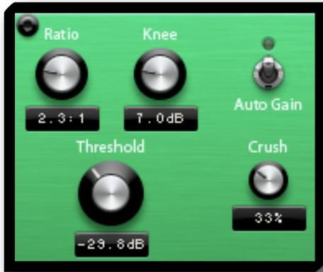
• **Threshold** - sets the level above which compression is applied
