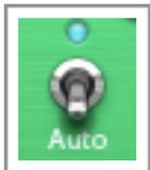
When the **Auto** switch is activated, the compressor 'Release' control becomes ineffectual, as the compressor release-time becomes automatic, varying according to the dynamics of the programme material. It should be noted that the release is not completely independent of the attack setting, as the compressor must compensate its release mechanism in different ways for fast and slow attack times. Thus the dynamics of the automatic release will differ according to the attack setting.
