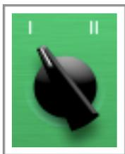
*There are two attack/release circuits to choose from. Type I provides a classic character more prone to signal-dependent distortions, while Type II offers a more pure (modern) detection, with less dependency on signal level and dynamics.*
