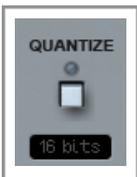
If the MaxLimit is used as a final stage mastering tool, the output can be quantized for the end medium by activating this button and setting the bit-depth accordingly (the depth can be set by clicking on the text display box below the *QUANTIZE* button and then selecting an appropriate option).
