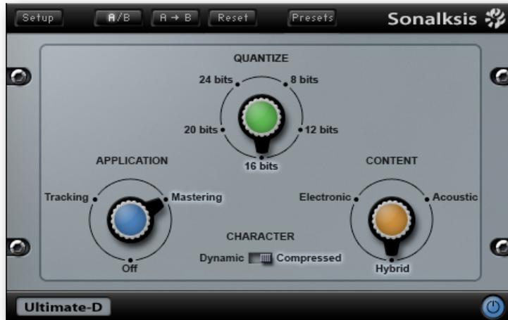
Ultimate-D is an end-chain mastering tool providing variable re-quantization using proprietary Sonalksis 'dither' and noise shaping functions for supreme digital resolution enhancement. The processor combines these advanced processing techniques with a unique interface that contains intuitive parameters, very unlike traditional re-quantisation processors.
