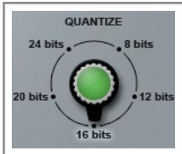
**Quantize** – this determines the output bit-depth, and should be set according to the resolution of the medium for which you are re-quantizing.
